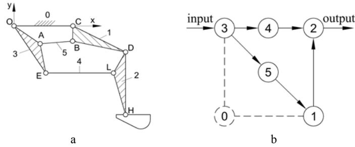
Fig 2. Kinematic diagram (a) and structural energy graph (b) of mechanisms type Stephenson I of die casting dosing robot "Feedmat 1"
