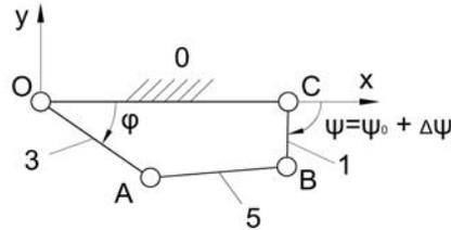
Fig. 3. Kinematic diagram of the control four-bar linkage
