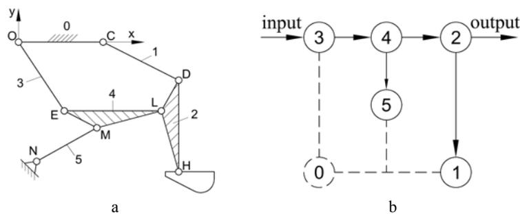
Fig 1. Kinematic diagram (a) and structural energy graph (b) of mechanisms type Stephenson III of foreign die casting dosing robots of the firms "Toshiba" and "Advance"
