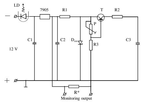
Fig.1. Electronic circuit for diade power supply: D<sub>200</sub> - zener diade, selected 5 V
