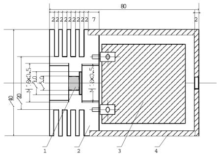
Fig.2. Mechanical structure of the laser imadiation: 1 - laser diode, 2 - cooling radiator, 3 - electronic supply driver, 4 - protective plastic cylinder
