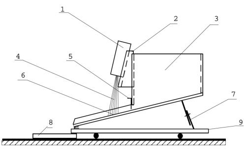
Fig.3. General mechanical pattern of "SOLAR-2" Laser system for pre-soving grain irradiation: 1 - laser irradiation comprising a semi-conductor laser, mounted in a
