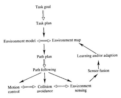
Fig. 2. Mobile robot control hierarchy, showing information flow
