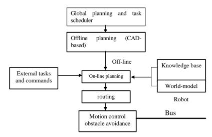
Fig. 4. Task planning of mobile robots
