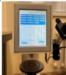
Figure 4.17 EBP BRV-187.5T hardness tester with mounted indenter used in the study.
