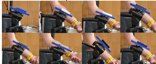
Figure 4.4. Photos from the experiment to determine the coefficient of sliding friction.
