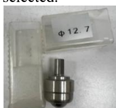
Figure 4.15 Indenter with a diameter of 12.7 mm
