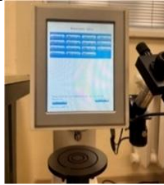
Figure 4.17 EBP BRV-187.5T hardness tester with mounted indenter used in the study.
