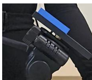
Figure 4.5 Photo from the experiment for determining the coefficient of sliding friction TPU+HIPS.
