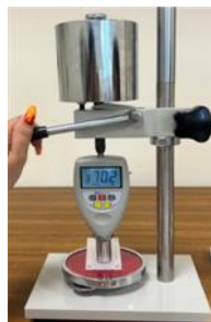
Figure 3.6. Shore microhardness measurement device (described in Chapter 2).
