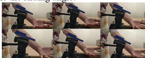
Figure 4.3. Images from the experiment to determine the coefficient of sliding friction
