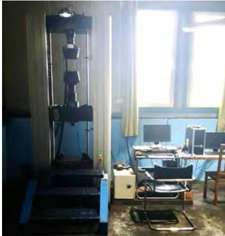
Fig. 1.16. Universal tensile strength machine WDW-300
