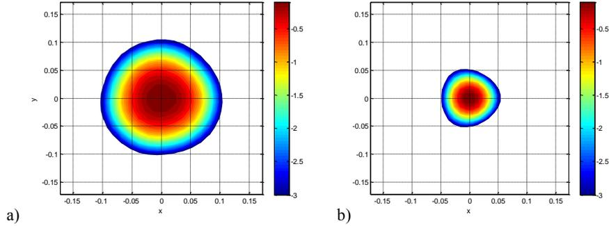
**Fig. 1.** Reconstructed by SONAH acoustic map of point source of a single-tone signal on the distance 10 cm: a) without interpolation b) with interpolation.
