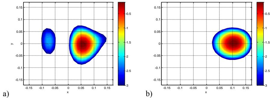
**Fig. 2.** Reconstructed by SONAH acoustic map of point source of the point source located in the point (0.1, 0) on the distance 10 cm: a) without interpolation b) with interpolation.
