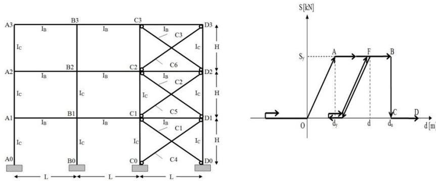
**Fig. 1.** The frame system and the constitutive law for the cable-elements.
