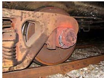
Fig 6. Overheated railway vehicle axle box (Hotbox)
