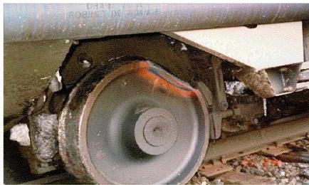
Fig 5. A flat spot occurred while the vehicle wheel set is dragging along the rail
