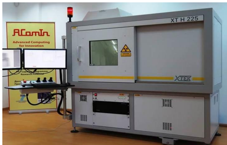
Fig. 1. Industrial CT scanning system, part of AComIn SmartLab equipment [2].
