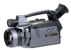
The FLIR P640 thermal imaging camera has an uncooled microbolometer detector that produces thermal images of 640 x 480 pixels. The FLIR P640 has some very useful built-in features that make it ideal for predictive maintenance, such as a laser pointer, Picture in Picture and FLIR Thermal Fusion to merge the visual and the thermal image.
