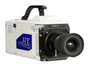
NAC's Memrecam HX-6 offers an astounding 5 MegaPixel resolution at up to 1,000 fps, Full HD resolution at up to 2,330 fps, 1 MegaPixel resolution at up to 4,600 fps, and much more. The HX-6 gives the user the best possible solutions: the highest resolutions available; the highest light sensitivity available; and ultra fast imaging.
