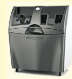
printing and operates with safe build materials, active dust control and zero liquid waste. Some of the ProJet 460Plus technical specifications are: resolution - 300 x 450 dpi, minimum feature size – 0.15 mm, layer thickness - 0.1 mm, input data file formats supported - STL, VRML, PLY, 3DS, FBX, ZPR. The ProJet 460Plus 3D printer
