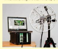
The Brüel & Kjær system for sound analysis allows merging/fusing of information from the different modality sensors - microphone array and camera. Acoustic Holography and Beamforming techniques are used for localizing sound sources. Two
