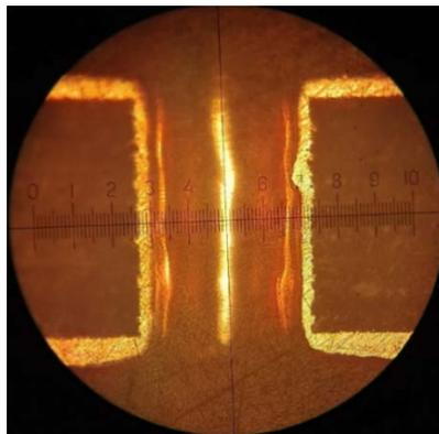
*Fig. 1 Cross section of the metallization vias*
