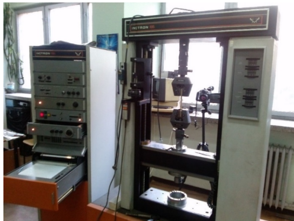
Figure.1. Press Instron 1195 testing tension and compression up to 10 tons.
