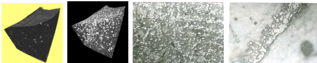
Fig 8. Flaw detection of articles of sintered boron carbide
