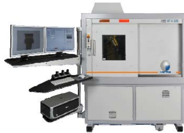
Fig. 5. Industrial 3D Tomograph
