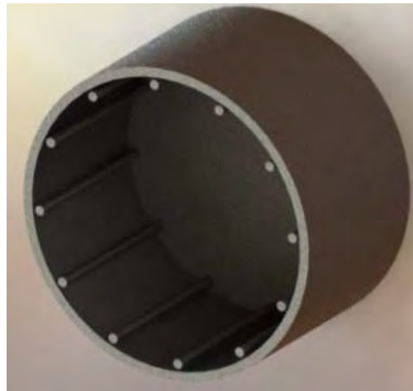
Fig. 5. 3D CAD model of the laboratory mill.
