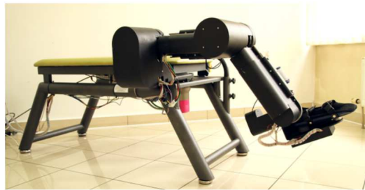
Fig.2. Robotized device for rehabilitation LEG-100
