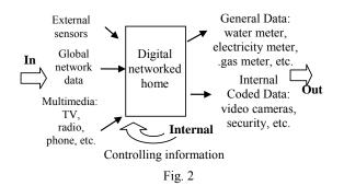
Using information from different inside and outside sensors as the internal ones in a feedback loop gives the possibility to achieve desired control conditions.
