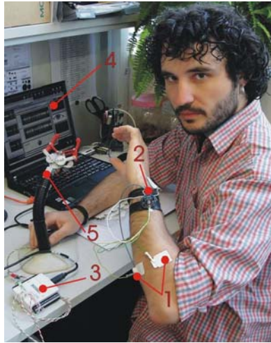
Fig. 6. Control of the electromechanical gripper by registration of the signals generated by movement of the palm
