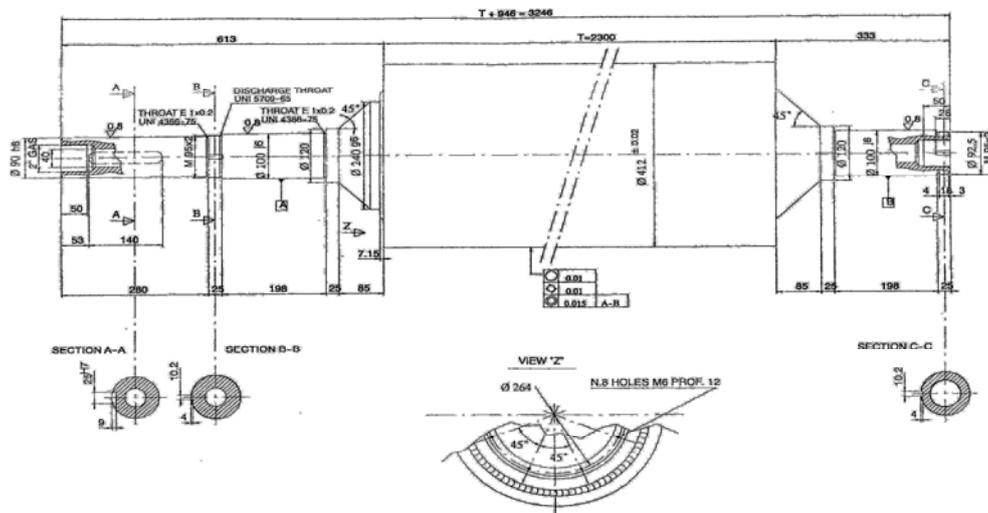
Fig. 1. Shaft for extruding sheet material
