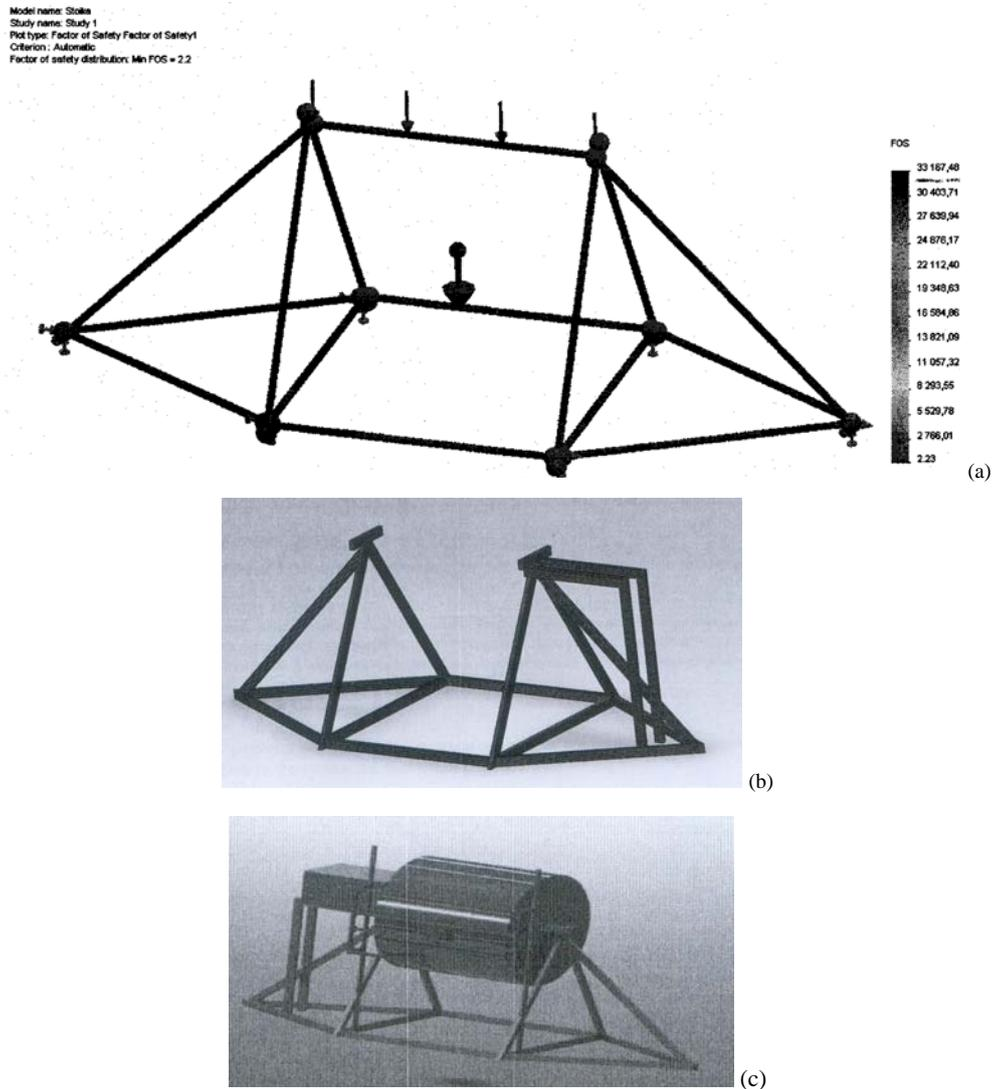
Fig. 5. The frame of the mechatronic systems for coating inspection: FEM analysis of the frame (a); CAD models of the frame (b) and (c)
