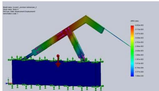
Fig. 3. Displacement of the manipulator made of Poly Carbonate material under the influence of actuator's force of 50 N
