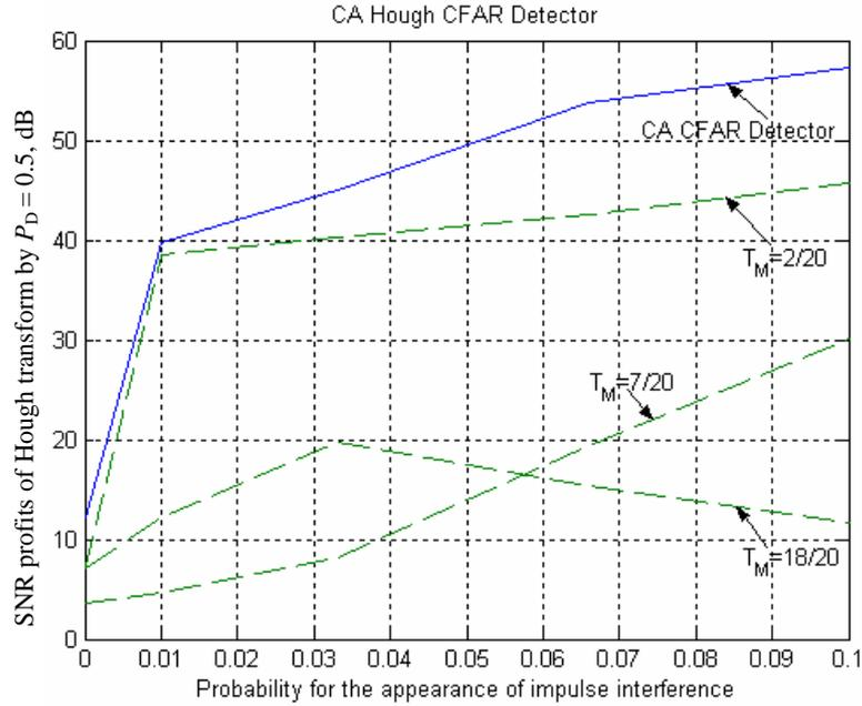
Fig. 5. Profits of a Hough detector (dashed line) with CA CFAR processor for 20 scans,  $T_M = 2$  and two optimal values of the detection threshold,  $T_M = 7$  for  $e_0 = 0$  and  $T_M = 18$  for  $e_0 = 0.1$ , compared to a CA CFAR detector (solid line) for  $N = 16$
