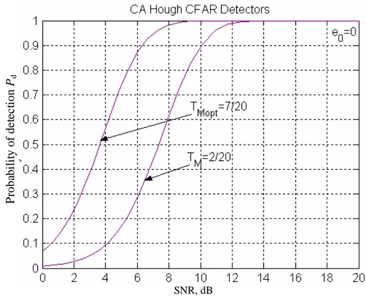
Fig. 3. Probability of detection of a Hough detector with CA CFAR processor in pulse jamming, for  $T_M=2$ ,  $T_M=7$  and  $e_0=0$
