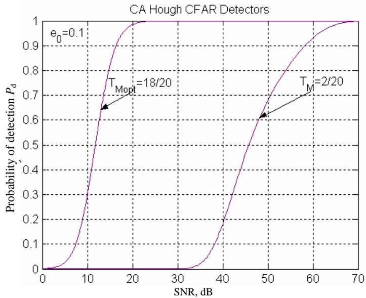
Fig. 4. Probability of detection of a Hough detector with CA CFAR processor in pulse jamming, for  $T_M=2$ ,  $T_M=18$  and  $e_0=0.1$
