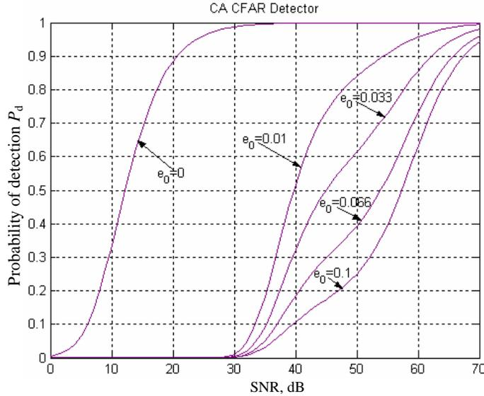
Fig. 1. Probability of detection of Cell Averaging Constant False Alarm Rate (CA CFAR) detector in the presence of pulse jamming, for  $P_{FA}=10^{-4}$  and  $N=16$
