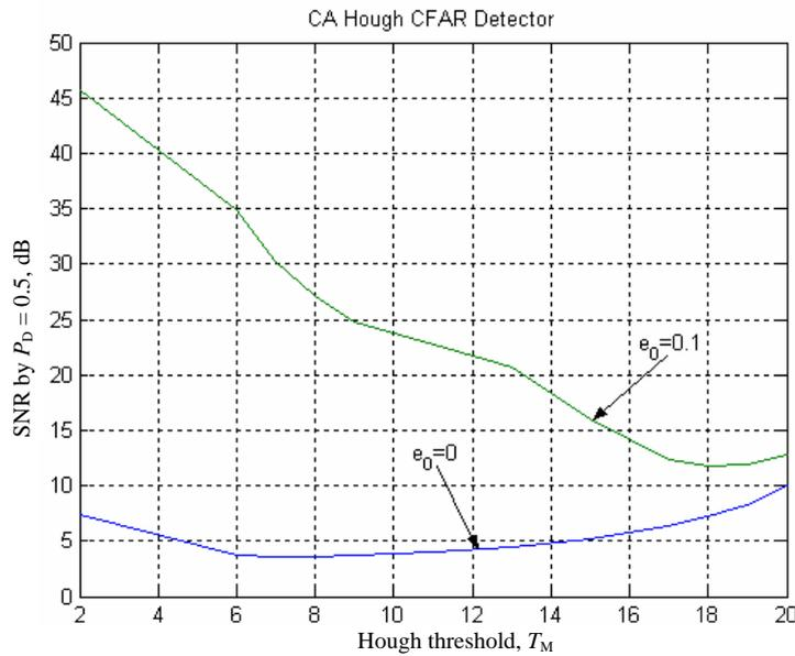
Fig. 2. Average detection threshold of a CA Hough CFAR detector
