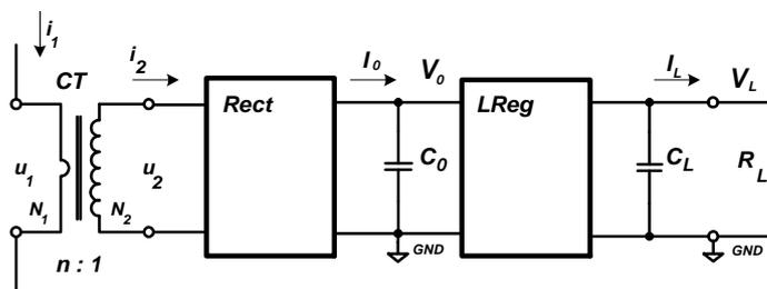
Fig. 1. Block-diagram of the proposed Current-to-voltage converter
