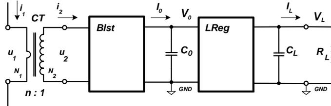
Fig. 6. Current-to-Voltage Converter, with controlled  $P_2$  exceed power rise
