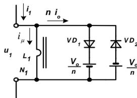
Fig. 2. Equivalent presentation of the Converter
