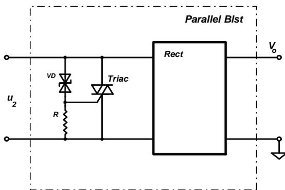
Fig. 7. Parallel-Type Ballast **Blst** – with Full-cycle control
