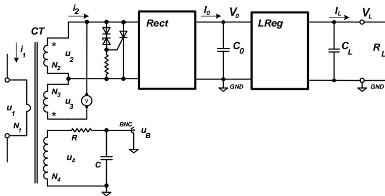
Fig. 9. Experimental Current-to-Voltage Converter
