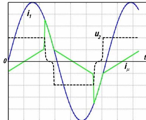
Fig. 5. Currents and voltages of a Converter, implemented on a Core with typical  $B(H)$  magnetizing loop
