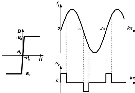
Fig. 4. Primary winding's Current  $i_1$ , Secondary Voltage  $u_2$ , and Core's Magnetizing curve  $B(H)$  of the Current Transformer  $CT$  at sub-critical conditions
