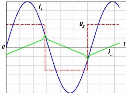
Fig. 3. Current transformer's voltages and currents  $I_{1min}$
