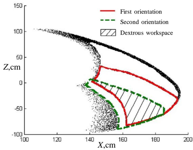
Fig.3. Workspace for the two fixed orientations
