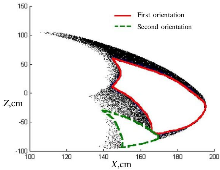
Fig.4. Workspace for the two fixed orientations
