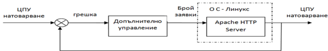
Fig. II.1. Structural scheme of the examined system
