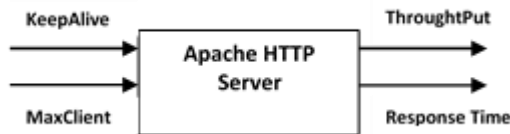
Фиг. III.2. Apache HTTP Server, presented as an automated control system
