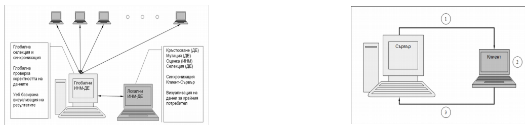
Fig. 2.1 Training system based on DE and ANN in a distributed environment (left) and sharing tasks in a distributed computing system (right).
