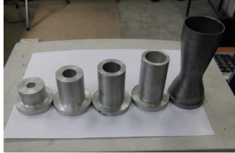
Fig. 3.3. Photo of rocket engines with different diameter of the critical section. From left to right: D_{\text{sect}} = 5 mm, 8 mm, 10 mm, 12 mm, 20 mm (engine is off). The impact speed is calculated according to formula (2.13). The theoretical value is 7.37 m/s (when R = 226\text{N} , m_1 = 9.12 kg), but the real speed is 6.8-7.0 m/s. In Regime 4 a high-velocity controlled impact is realized
