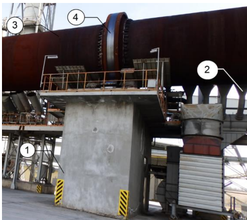
Fig. 4.3. Furnace, 1 – base, 2 – coolers, 3 – furnace, 4 – bearing
