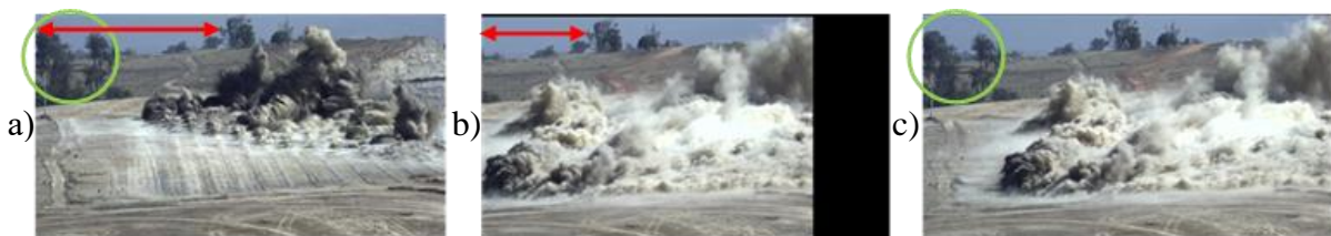
Fig. 33. Stabilization of a video clip, containing a record of controlled explosion: a) first frame; b) last frame after stabilization in “a point”; c) last frame after stabilization on a smooth trajectory.
