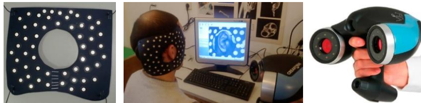
Fig. 5. a) The cartoon "helmet"; b) A person under scanning; c) VIUscan 3D scanner
